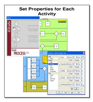
To set Properties for an activity, double clicking the activity on the Process Diagram opens a window wherein Resources, Task Durations, and Output Characteristics can be Set. Here are some of the Resources for SeaCage(1): 1 Center Manager, 35 days of Sea Vessel, 90 metric tons of Feed Pellets, etc.
